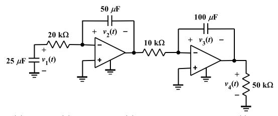
Given  $v_1(0) = 20 \text{ V}$ ,  $v_2(0) = -10 \text{ V}$  and  $v_3(0) = -5 \text{ V}$ , use LTspice to plot  $v_4(t)$  for  $t \ge 0$ . Use the model shown below to build a subcircuit model for the OpAmps.
